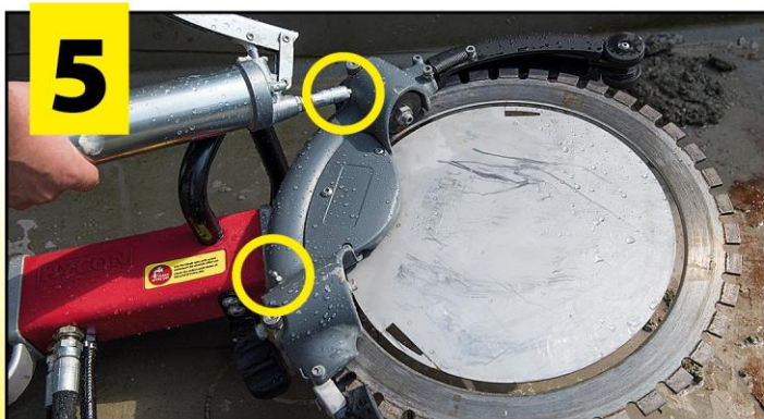
Apply grease to all four grease fittings.
