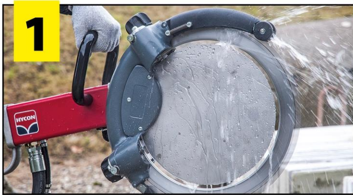
Let the ring blade spin free for minimum 30 seconds after EACH JOB. Clean water will flush the rollers.
