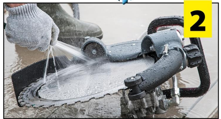
Clean the rollers and housing very carefully with the water hose EVERY DAY after use...
